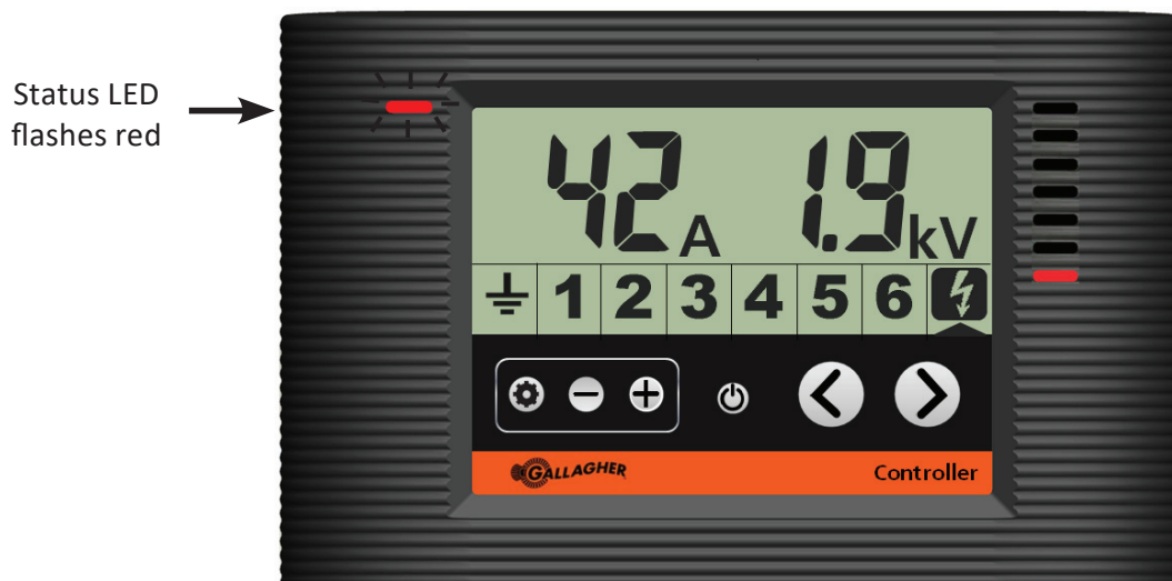
Controller showing the energizer in output alarm
