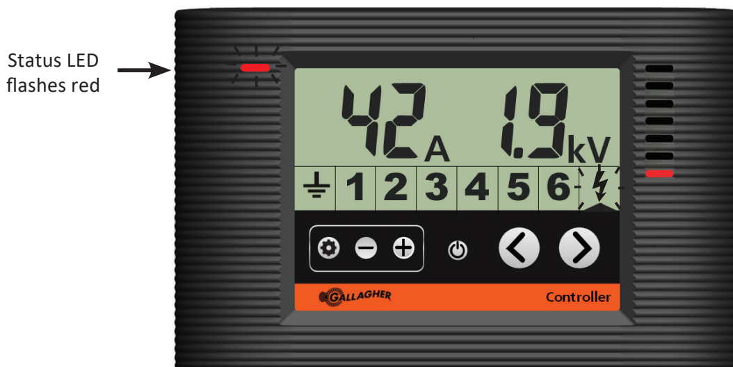
Controller showing the energizer in current alarm
