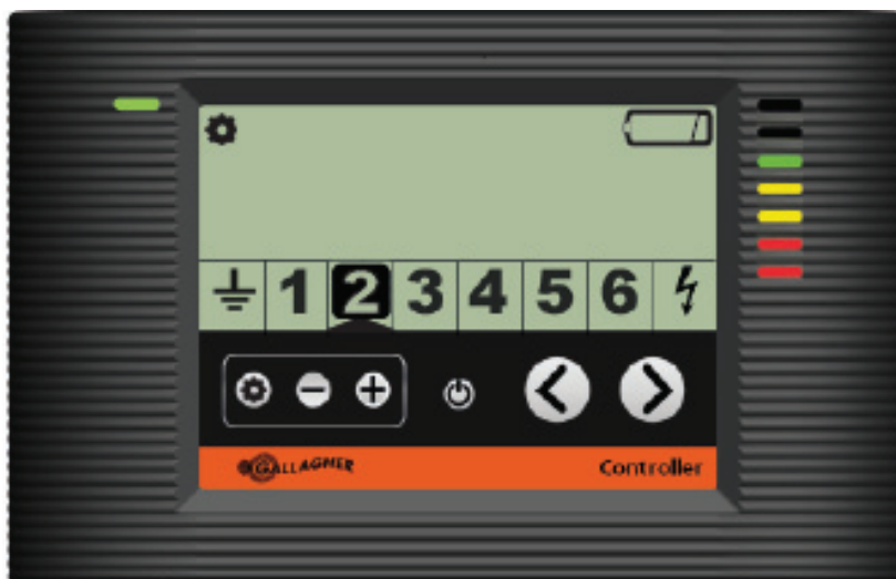
Controller showing zone 2 with a low battery
